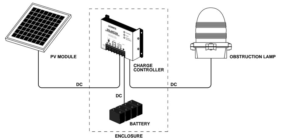
This system is controlled by the charge controller that control charging current from solar panel to storage battery and supply to obstruction lamp at night or when insufficient sunlight for 30 minutes.
