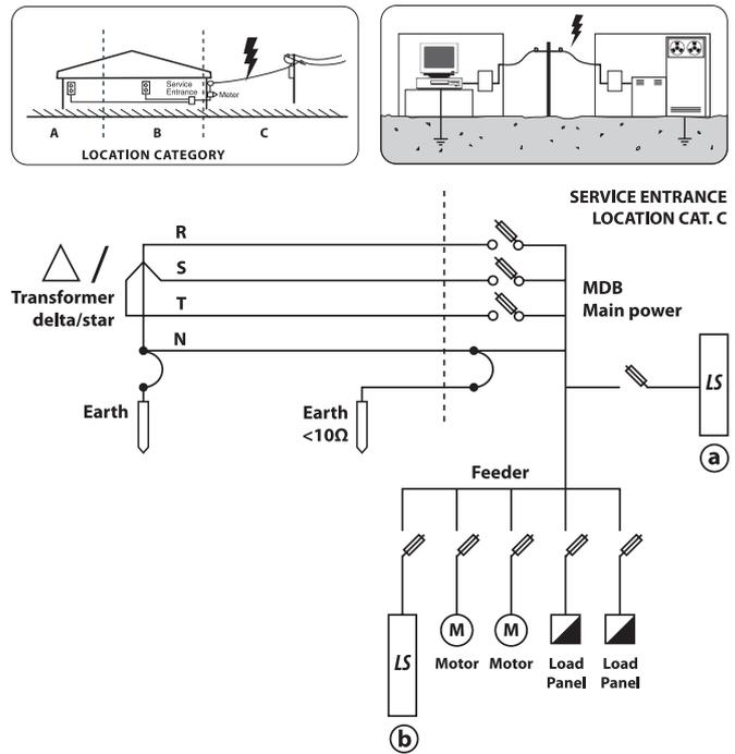
4.4.2 **Surge source installation:** Install Surge Diverter at load distribution or load panel to protect surge from the start-stop equipment or in the special protection areas such as signal control room and server room.
