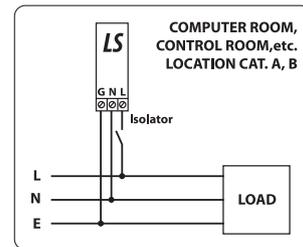
4.5 Recommend to install a circuit breaker to separate Surge Diverter from electrical system for maintenance and protection of the cables from the surge diverter to the electrical system.
