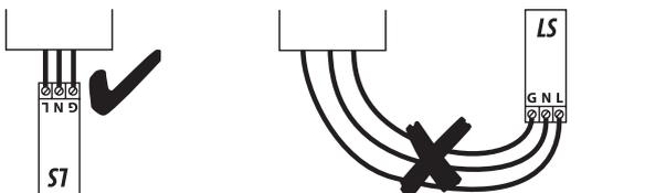
4.3 In case that it is not possible to wire the system with 25 cm. cable length, use two sets of 4 mm<sup>2</sup> cables which each length is shorter than 50 cm. Split them into 2 sets (L, N and E) with minimum space 10 cm. or 4 inches. Tie the cables with cable tie or spiral wrap for the whole length.
