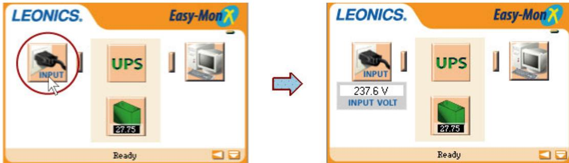
Figure 7 How to view AC input voltage
