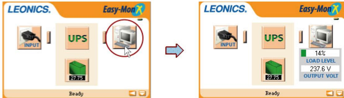
Figure 9 How to view AC output volt and load level
