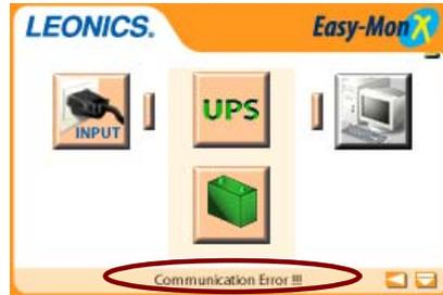
Figure 13 Communication error warning
